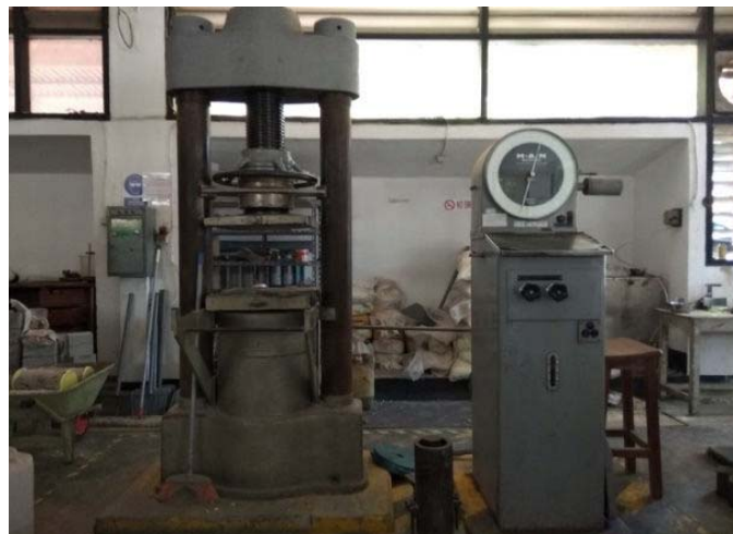
Figure 3. Compressive Testing Machine.
